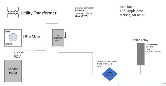
The Total Generator Nameplate AC Rating (kW): Is calculated by the number of inverters multiplied by the inverter power rating (kW\_AC) per inverter.
